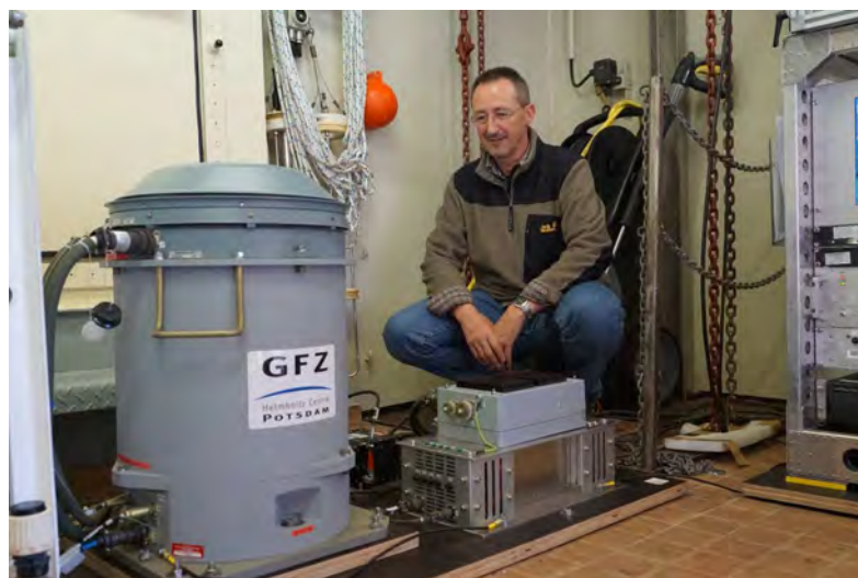
Gravity meter (Chekan) installed on board DENE B
