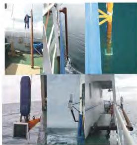
Fig. 2. Installation of the "SES-2000 standard" and "Hydra" transducers on board of vessel.
