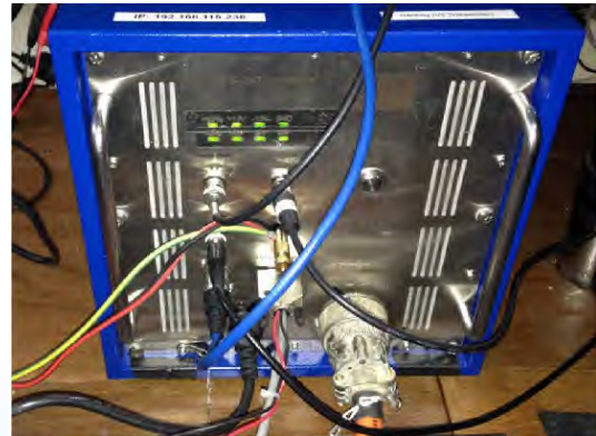
Parametric echosounder main unit with used all input/output sources.
